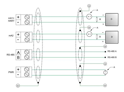
Figure 3-2: Wire power and outputs in a HART single-loop environment
