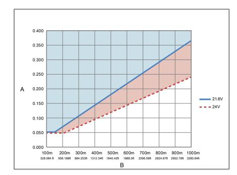
Figure 1-2: Minimum wire area (mm<sup>2</sup> per meter or foot)
