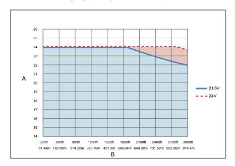
Figure 1-1: Minimum wire gauge (AWG per foot or meter)
