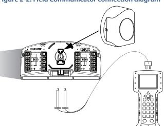
Figure 2-2. Field Communicator connection diagram
