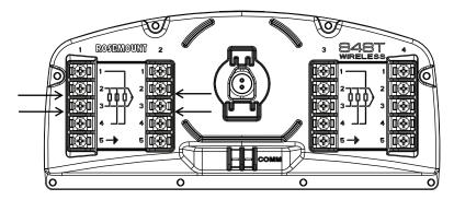
2. Angle adapter and slide spade lugs into terminals 2 and 3 on the left side, as shown in the figure below. Ensure that the positive and negative polarity indicators match on the adapter and the terminal block.
