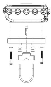
3. Run wiring (and conduit, if necessary) from the sensor to the 848T. For an easier installation, use the outside conduit entries, as shown below. Any unused conduit entries should be sealed with an approved sealant using the included threaded conduit plug.
