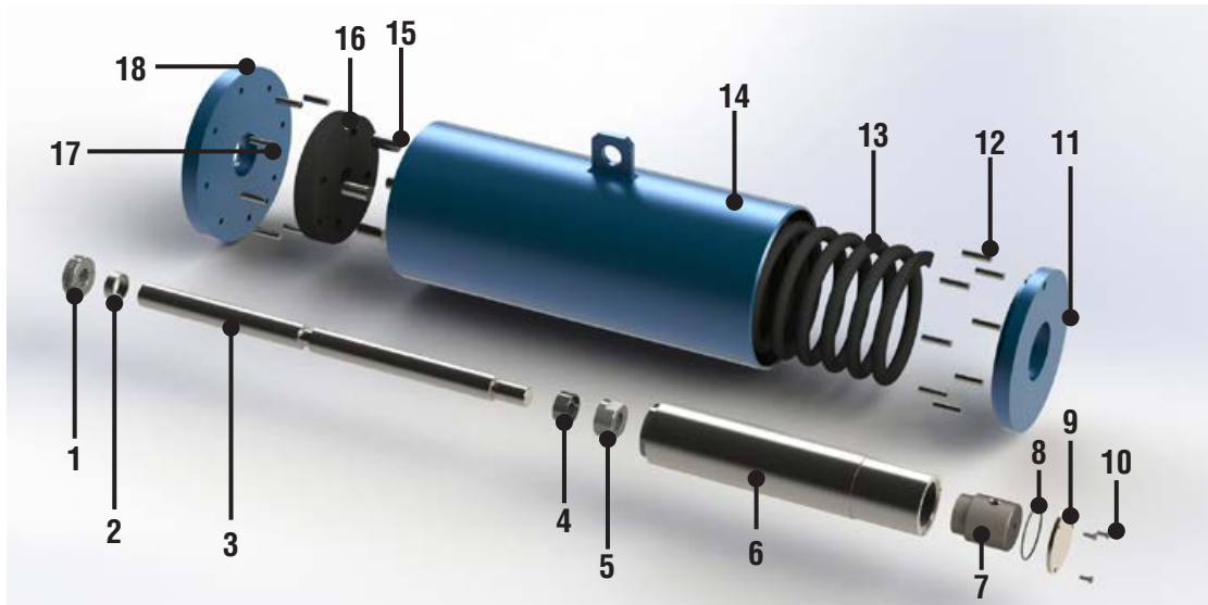
Figure 22: Spring Can Exploded View
