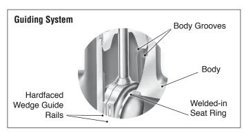
The body groove extends high in the body neck region, so that in the open position the wedge assembly is both trapped and fully guided. Body grooves are hardfaced for critical service valves.
