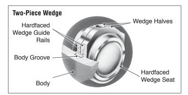
The outstanding design feature of the Equiwedge gate valve is unique two-piece wedge that permits maximum independence and flexibility for good sealability and freedom from sticking.
