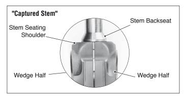
The Equiwedge two-piece wedge design allows the use of a space and weight-saving "captured stem."
