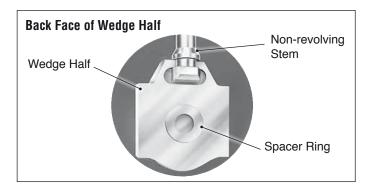
Wedge halves are separated the proper amount by a spacer ring that provides controlled deflection from stem loading. Use of a space and weight-saving "captured stem" (shown here and in Figure 4) is possible because of the two-piece wedge design.
