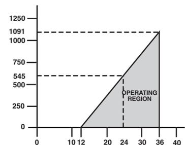
$$V_{min} = 12V + [.022A \cdot (R_L)]$$
