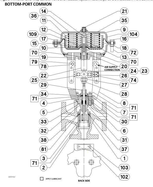
Figure 11. Fisher GX 3-Way Control Valve and Actuator System Assembly, Fail-Down, Bottom-Port Common
