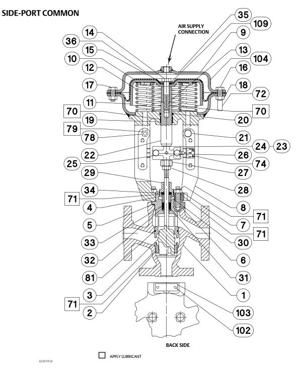
Figure 8. Fisher GX 3-Way Control Valve and Actuator System Assembly, Fail-Up, Side-Port Common
