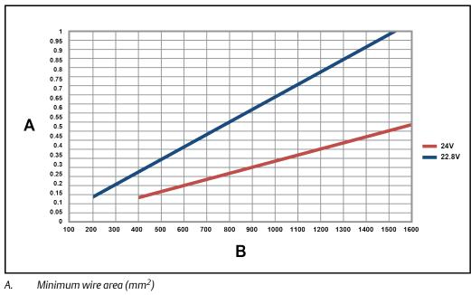
Figure 1-4: Minimum wire area with 300  $\Omega$  barrier
