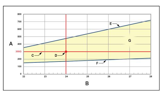
Figure 1-5: Limits of series resistance versus supply voltage
