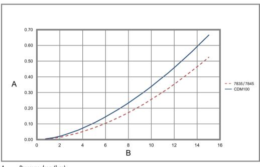
Figure 1-2: Sample pressure drop calculations (fluid viscosity equals 10 cP)
