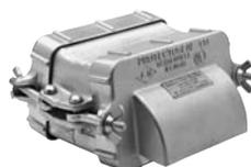
End-of-Line Deflagration Flame Arrester provides protection of the tank's vapor space if an ignition source is introduced outside of the tank. Suitable for NEC Group D (IEC Group IIA) vapors.
