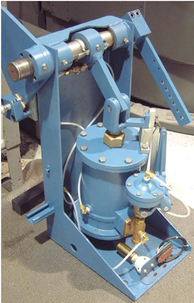
*Remanufacturing drives include new piston rods, seals, gaskets, piston cups, springs and tubing.*
