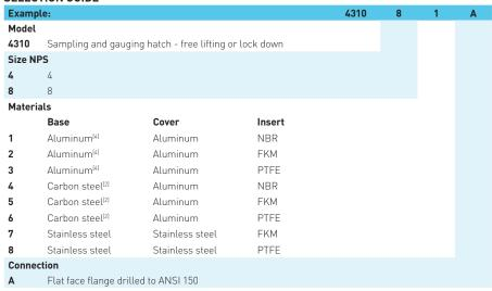
**Example:** Model Number 43108A is a 4310 Series sampling and gauging hatch with 8" aluminum base and cover, NBR insert, flat face flange drilled to ANSI 150.
