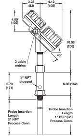
7xM / 7xN with flushing connection
