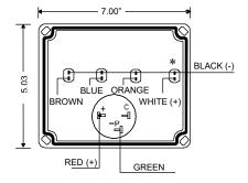
\* WARNING LABEL PLACED HERE: Warning: Low Voltage Inputs Only
