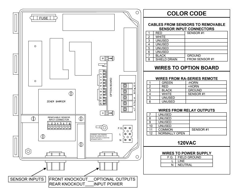
NOTE: To maintain proper shielding, <u>BLACK **sensor** wires</u> and SHIELD DRAINS <u>should</u> <u>**not** be connected together</u> at sensors.
