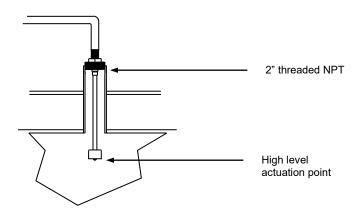
Connection of the sensor to the control unit cable is made in a junction box. For detailed wiring scheme refer to appropriate drawing (see pg.7 and 8). These connections must be made using supplied SK-4 connector sealing kit.
