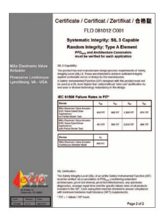
Additionally, the MXa achieved a SIL rating for the actuator including all of the standard controls such as status contacts and torque sensing. Failure in time (FIT) metrics are improved when a partial stroke test is utilized (PST). Refer to the table below.
