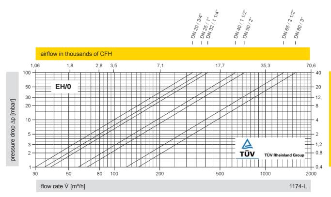
The flow capacity chart has been determined with a calibrated and TÜV certified flow capacity test rig. Volume flow  $\dot{V}$  in [m³/h] and CFH refer to the standard reference conditions of air ISO 6358 (20°C, 1bar). Conversion to other densities and temperatures refer to Vol. 1: "Technical Fundamentals".
