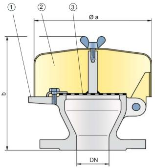
The vent cap PROTEGO® EH/0 main components are a housing (1), a weather hood (2) and a protection screen (3). The device is equipped with a fixed weather hood out of metal. The protection screen prevents particles or rain from entering the line.
