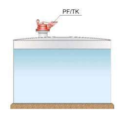
Gauge Hatches can be applied on tanks with floating roof.
