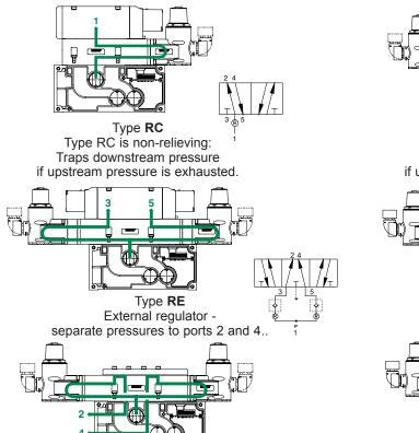
Type RD Dual pressure from a single supply.
