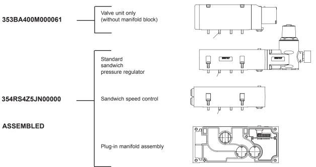
Note: Sandwich speed controls can only be used with single sandwich pressure regulators.
