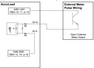
For pulse transmitters requiring 12 VDC (such as GPST), install the P2412 converter. See the AccuLoad Preset Accessory P2412 Converter Installation manual (MN06117) for details.
