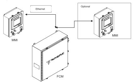
The FCM unit can be installed at a location that is convenient to service personnel. The MMI units can be installed for convenient access by drivers. Typical installation approaches are shown below.
