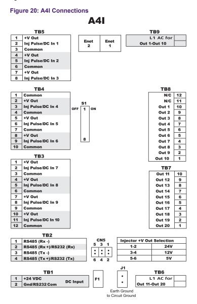
The A4I board has jumpers that allow customization. If the A4I board is connected to additive meters for which the transmitters require DC power, the voltage select jumpers (see Table 14: A4I Jumper Settings) are used to set the meter power supply voltage to 5, 12, or 24 VDC.
