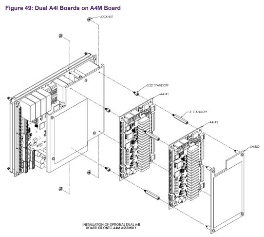
Complete the following steps to install one or two A4I boards onto the AccuLoad IV's A4M board:
