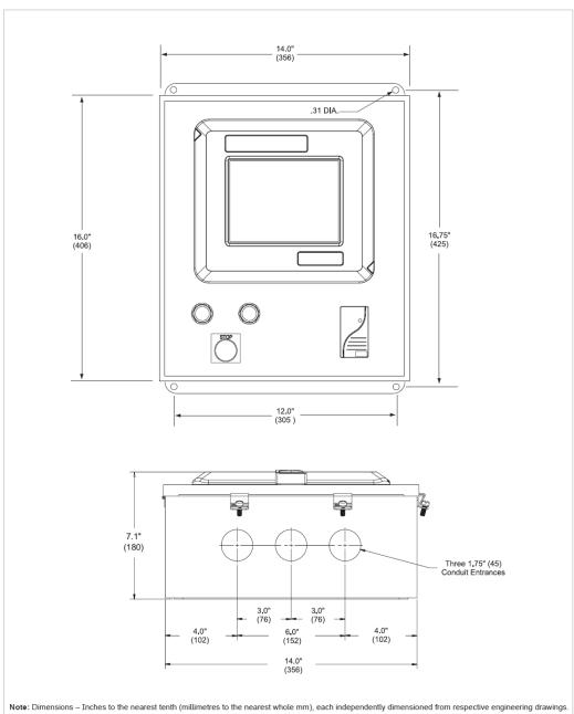
Figure 6: AccuLoad IV N4 and MMI Dimensions
