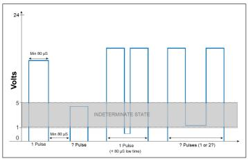
Figure 25: Meter Pulse Requirements
