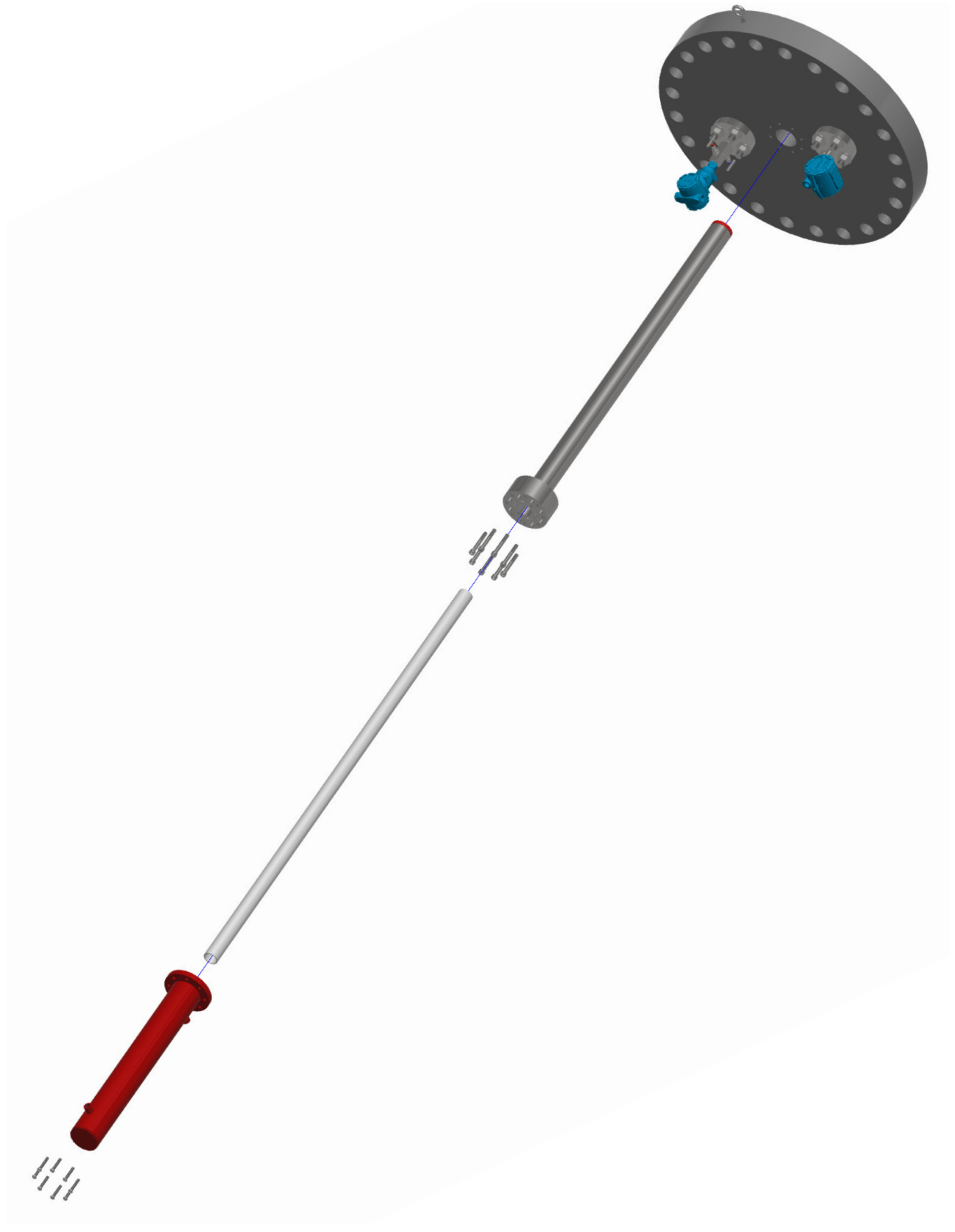
Figure 5.7 - Remove Stop Assembly Tube
