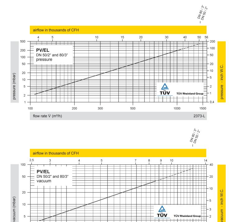
The flow capacity charts have been determined with a calibrated and TÜV certified flow capacity test rig. Volume flow V in (m³/h) and CFH refer to the standard reference conditions of air ISO 6358 (20°C, 1bar). Conversion to other densities and temperatures refer to Vol. 1: "Technical Fundamentals".
