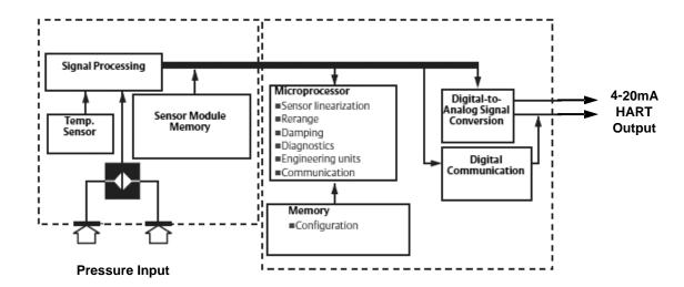
Figure 1 - Rosemount 3051 Pressure Transmitter Block Diagram
