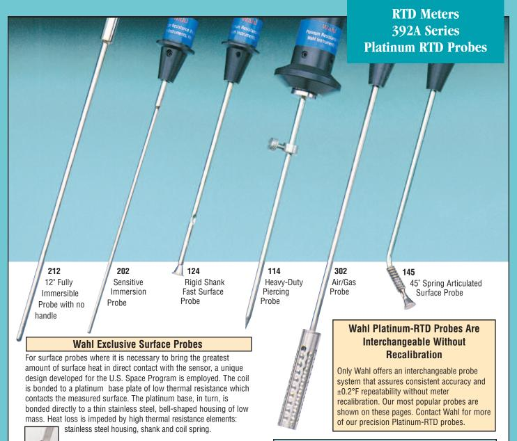
The coil spring in Wahl 121 and 145 surface probes provides automatic articulation of the tip for conformity and uniform contact with the surface being measured. This is especially useful in blind recesses where contact measurements are made by "feel" instead of sight.
