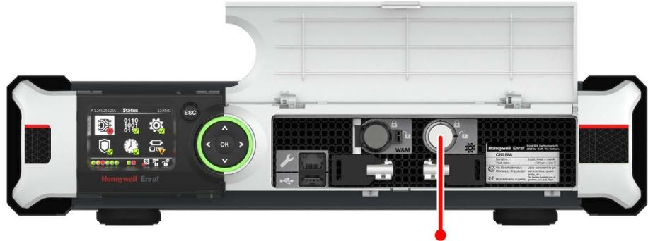
FIGURE 5-9 CIU 888: Configuration lock key switch
