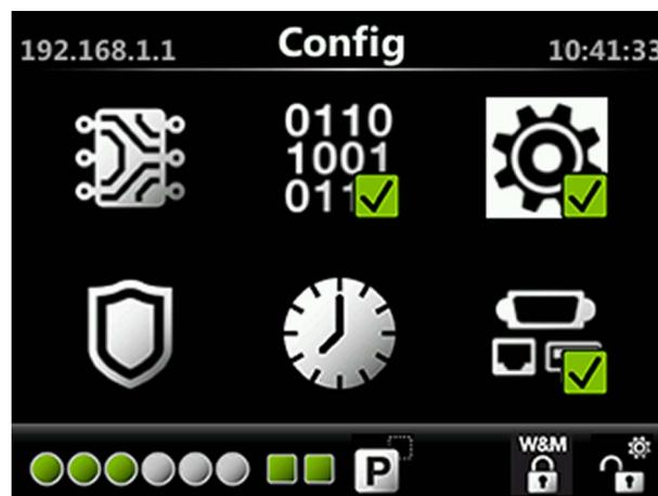
FIGURE 5-10 Status Dashboard: configuration settings are unlocked
