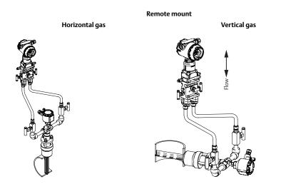
Figure 6. Flowmeter Orientation for Steam
