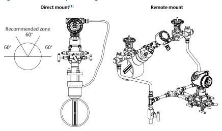
For wet steam, do not mount the flowmeter at the direct vertical position. Mounting at an angle will avoid measurement inaccuracy due to water running along the bottom of the pipe.
