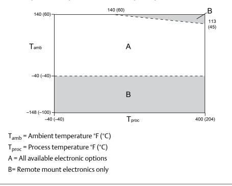
Ambient and process temperature limits for Super Duplex ELITE meters
