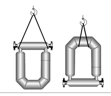
Figure 2-2: Center of gravity for large meters
