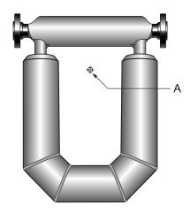
A. Typical center of gravity
