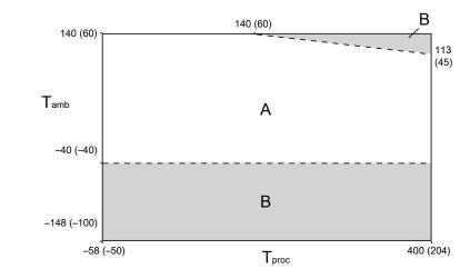
Ambient and process temperature limits for ELITE CMFS007, CMFS025–CMFS150 meters
