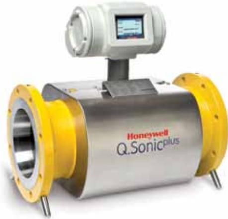
The patented path configuration—a fully symmetrical layout of four swirl paths with double reflection and two single reflection paths—enables the measurement of both swirl and asymmetry, resulting in previously unequalled profile recognition and diagnostic possibilities.
