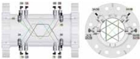
The Q.Sonic<sup>plus</sup> uses two pairs of double and two single reflection paths. Taking the mean value of both pairs will result in a symmetrically weighted measurement.
