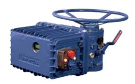
The L120 is factory-lubricated, suitable for weatherproof service in temperatures ranging from -40°C (-40°F) to 65°C (150°F), as well as explosion proof and temporary submersion applications. Weatherproof enclosures meet NEMA 4 standards, as well as NEMA 6, IP67, and IP68 submersible standards. Explosionproof actuators meet Factory Mutual and Canadian Standards Association requirements.
