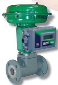
The 24000CVF/SVF is available in 316L (CF3M) stainless steel or WCC carbon steel materials. End connections are ASME CL150RF or CL300RF and PN 10-40 flanged.
