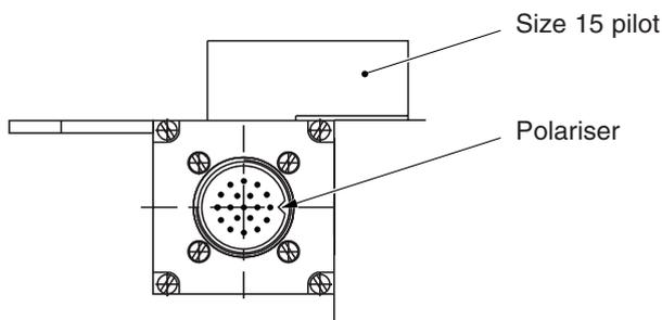
The unit is grounded with pin 12 of the connector. Grounding for personal protection is effected directly on the island with the ground hole ØM4.
