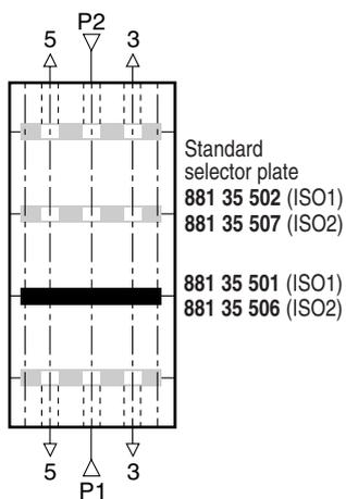
To obtain this configuration, it is necessary to procure one selector plate blanking flow paths 1, 3 and 5.
