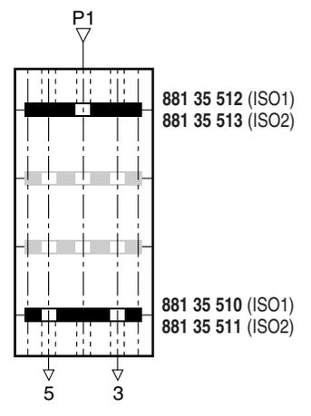
The use of one selector plate leaving flow path 1 open as well as one selector plate leaving flow paths 3 and 5 open at the endplates makes it possible (in the ISO 1 case) to obtain the above configuration without having to plug the ports.
