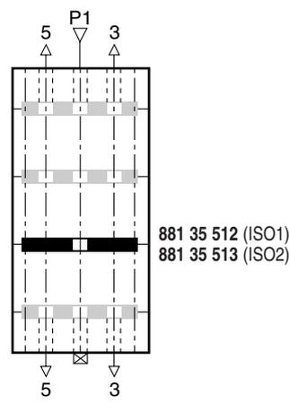
To obtain this configuration, it is necessary to procure one selector plate leaving flow path 1 open. This makes it possible to isolate the exhaust while retaining the common pressure supply. Fit a plug on the other end.
