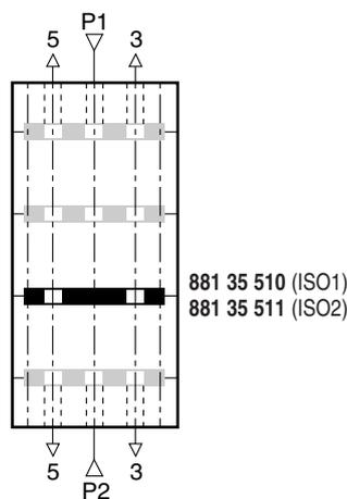
To obtain this configuration, it is necessary to procure one selector plate leaving flow paths 3 and 5 open.
