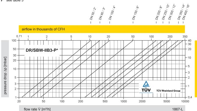
The flow capacity charts have been determined with a calibrated and  $T\ddot{U}V$  certified flow capacity test rig. Volume flow  $\dot{V}$  in [m³/h] and CFH refer to the standard reference conditions of air ISO 6358 (20°C, 1bar). Conversion to other densities and temperatures refer to Vol. 1: "Technical Fundamentals".
