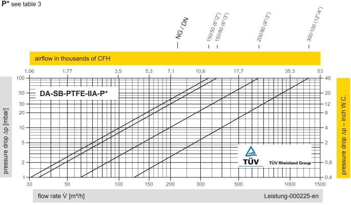
The flow capacity chart has been determined with a calibrated and TÜV certified flow capacity test rig. Volume flow V in [m³/h] and CFH refer to the standard reference conditions of air ISO 6358 (20°C, 1bar). Conversion to other densities and temperatures refer to Vol. 1: "Technical Fundamentals".
