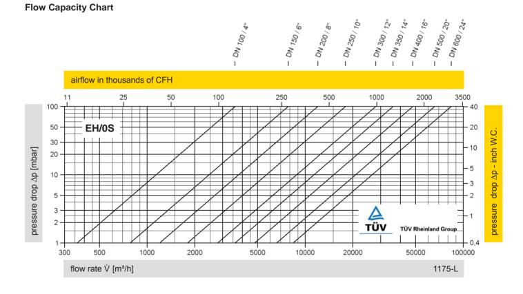
The flow capacity chart has been determined with a calibrated and TÜV certified flow capacity test rig. Volume flow  $\dot{V}$  in [m<sup>3</sup>/h] and CFH refer to the standard reference conditions of air ISO 6358 (20°C, 1bar). Conversion to other densities and temperatures refer to Vol. 1: "Technical Fundamentals".
