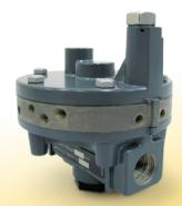
Volume Booster -Used in conjuction with a positioner on a throttling control valve to increase stroking speed. Connectors and piping can be installed for diagnostic testing.
