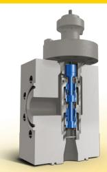
Cavitating Dirty Flow, Customized - Dirty Service Trim (DST) provides cavitation-control for applications with entrained particulate. It uses a combined axial and radial flow path that features large openings allowing particulate up to 19 mm (¾-inch) in diameter to pass through the valve.
