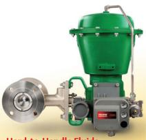
Hard-to-Handle Fluids -Fisher V500 and CV500 control valves offer low operating torque and combine the ruggedness of a globe valve with the efficiency of a rotary valve. Well suited to erosive, coking and other hard-to-handle fluids.
