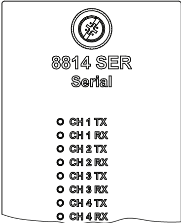
Figure 7-3: 8814 Serial Module LED Indicators
