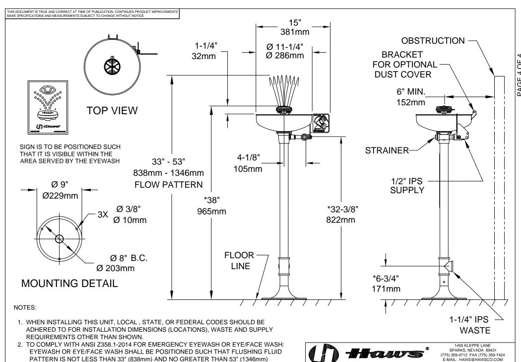
WEBSITE: WWW.HAWSCO.COM FROM SURFACE ON WHICH USER STANDS; AND 6.0" (153mm) MINIMUM FROM WALL OR NEAREST OBSTRUCTION. 7261-7271 3. \* DIMENSIONS MAY VARY BY ±1/2" (13 mm).
