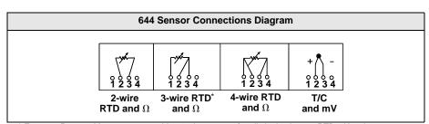
\* Emerson Process Management provides 4-wire sensors for all single element RTDs. Use these RTDs in 3-wire configurations by leaving the unneeded leads disconnected and insulated with electrical tape.
