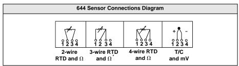
Rosemount Inc. provides 4-wire sensors for all single element RTDs. You can use these RTDs in 3-wire configurations by leaving the unneeded leads disconnected and insulated with electrical tape.
