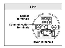
Figure 4-1. Transmitter Power, Communication and Sensor Terminal Figure 4-2. Typical connection of a Profibus configuration host to a transmitter loop
