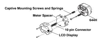
Use the following procedure to install the meter.
