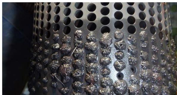
*Magnetite is a common iron oxide mineral with natural magnetic properties. Over time, it filled the flow passages of the valve cage, causing problems for the power plant.*
