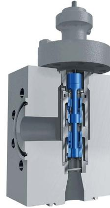
*Fisher Dirty Service Trim utilizes a series of flow restrictions and expansions to eliminate cavitation while allowing particulates up to 19 mm (3/4 inch) in diameter to pass through without plugging. Its design addresses pressure drops in the early stages and results in more efficient operation.*
