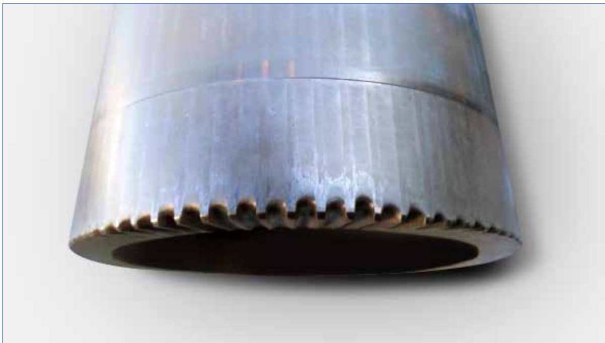
Damage to the control valve plug caused by steam leakage while closed.
