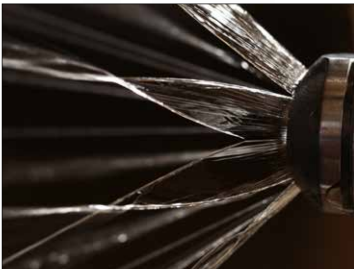
Spray pattern of a damaged mechanically atomized spray nozzle.
