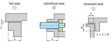
The dimensions given depend on the seal and volume of the enclosure and gas groups. Example: with a seal length L=12.5 mm and an enclosure volume  $\leq 100$  cm<sup>3</sup>, the MESG "i" will be:
