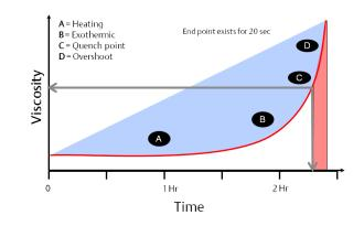
Illustration of the polymerization reaction, showing viscosity in relationship to time
