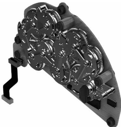
Figure 6.2 – Absolute Position Encoder
