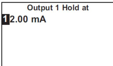
6. Enter the desired simulated output current.
