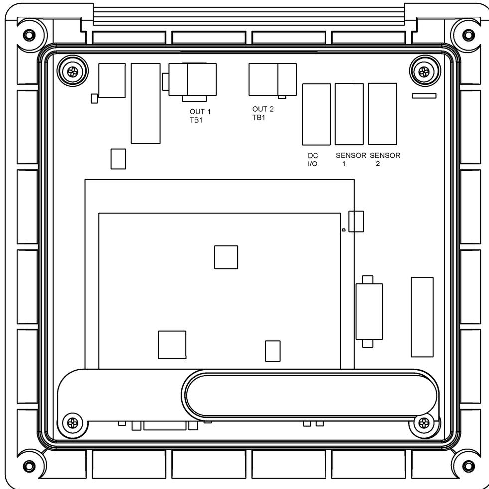
The analog outputs are on the main board near the hinged end of the enclosure door.
