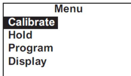
2. To assign values to the analog outputs, you must open the **Program** sub-menu. Use **Down** to move the cursor to Program. Press **ENTER**.
