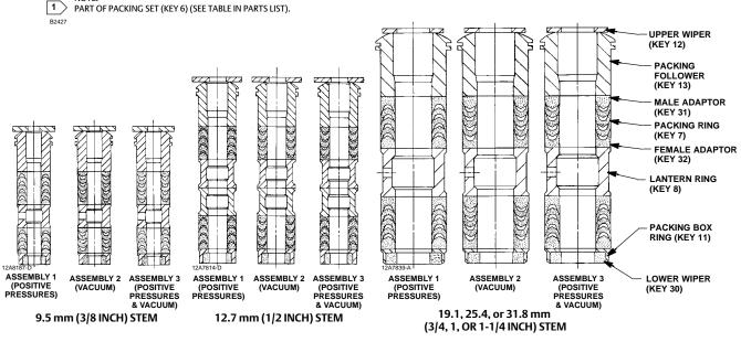
Figure 4. PTFE Packing Arrangements for Use in ENVIRO-SEAL Bellows Seal Bonnets
