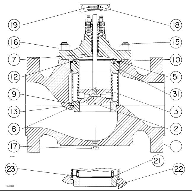
Figure 16. Fisher ES Valve Assembly with WhisperFlo Cage with Optional Drain Plug
