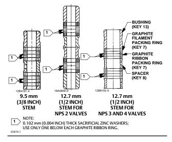
Figure 7. Detail of Graphite Ribbon/Filament Packing for Plain and Extension Bonnets
