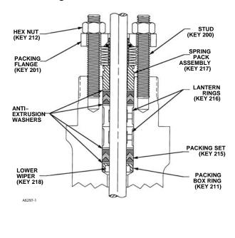
Figure 12. Typical ENVIRO-SEAL Packing System with Duplex Packing
