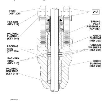
Figure 10. Typical ENVIRO-SEAL Packing System with PTFE Packing
