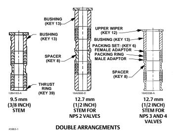
4. Loosen the packing flange nuts (key 5, figure 8) so that the packing is not tight on the valve stem. Remove any travel indicator parts from the valve stem threads.
