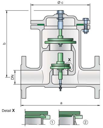
Tank connection depends upon flow capacity, set pressure and set vacuum for in- and outbreathing
