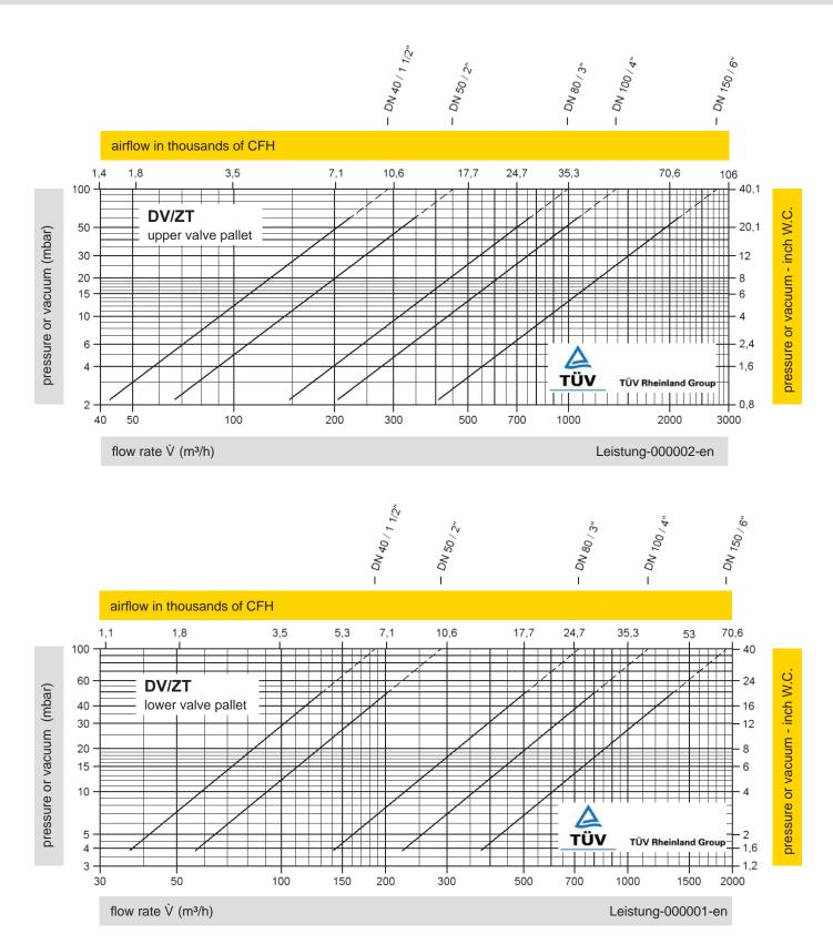
The flow capacity charts have been determined with a calibrated and  $T\ddot{U}V$  certified flow capacity test rig. Volume flow  $\dot{V}$  in (m³/h) and CFH refer to the standard reference conditions of air ISO 6358 (20°C, 1bar). Conversion to other densities and temperatures refer to Vol. 1: "Technical Fundamentals".
