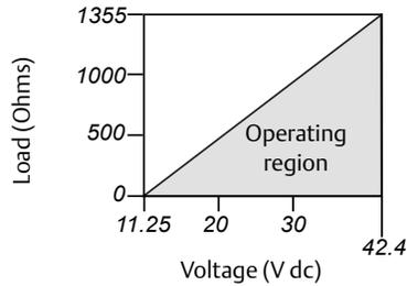
\*Communication requires a minimum loop resistance of 250 ohms.
