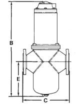
DA-3-150 thru D-6-150 Combination Strainer/Air Eliminator
