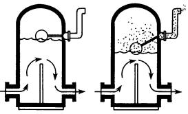
Once displaced to a predetermined point, a floatoperated valve opens and the accumulated air and
