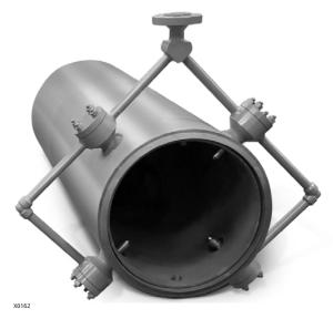
TBX-T—The TBX-T desuperheater incorporates a spraywater manifold of variable geometry Type AF nozzles that produce an optimized spray pattern over a wide operating range. These nozzles are strategically placed to achieve optimal mixing and quick vaporization at all flowing conditions (see figure 3).
