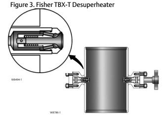
Figure 4. Detail of Spray Nozzle
