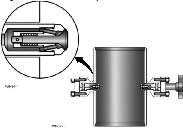
Figure 4. Detail of Spray Nozzle
