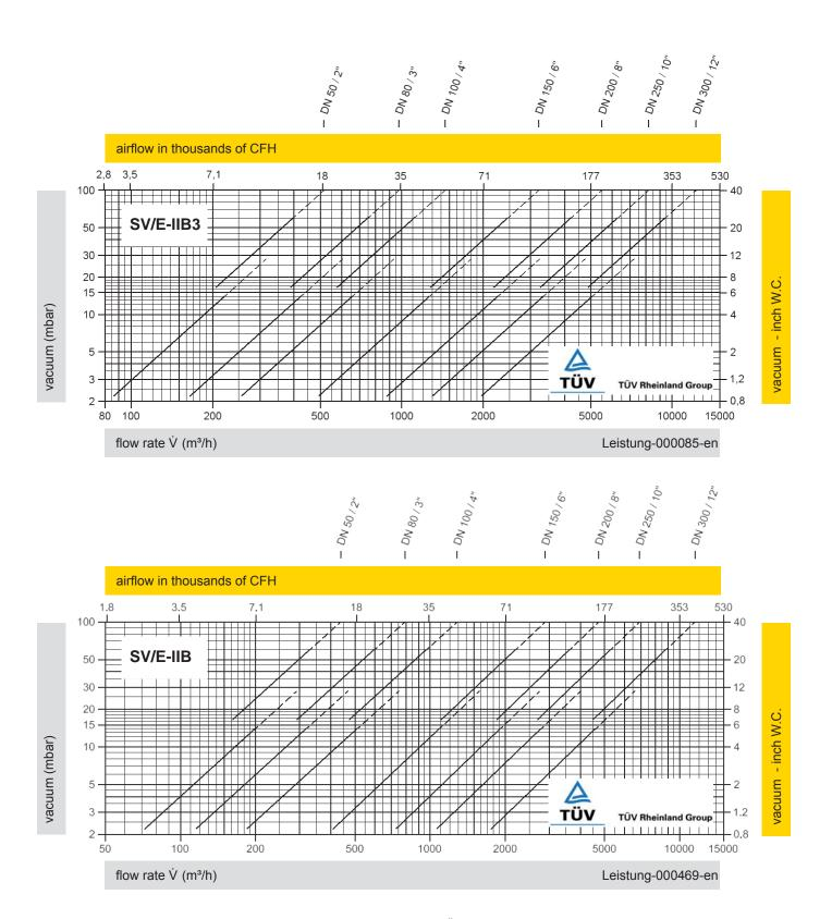
The flow capacity charts have been determined with a calibrated and TÜV certified flow capacity test rig. Volume flow  $\dot{V}$  in (m³/h) and CFH refer to the standard reference conditions of air ISO 6358 (20°C, 1bar). Conversion to other densities and temperatures refer to Vol. 1: "Technical Fundamentals".
