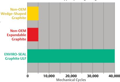
Non-OEM graphite packing does not measure up to the ENVIRO-SEAL graphite ULF packing system as proven by 2001 Emerson lab testing at 1500 psi and thermal cycling to 600°F without packing adjustment.
