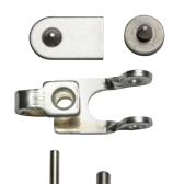
Babbitt Masterlinks are used with weldless chain to connect the two ends during installation of the chainwheel. The Masterlink returns the chain to its original load bearing strength with a quick and easy process. When a Masterlink is added to an order, the chain is prepared in our facility to eliminate the need for cutting or alteration on site.
